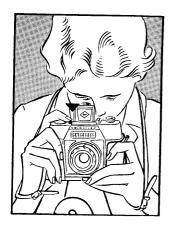
Another point in favour of the hood type of viewfinder is that you can aim the camera up in the air or downwards without twisting your body in any way. By using the sling you can also photograph satisfactorily in a crouching position. The Colorflex can even be used for photographs in crowds by holding it over your head and viewing the subject on the ground-glass screen from below.
