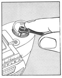
The flashgun, of the Agfa Synchro KM or Agfalux type, is first attached to the shoe of a flash bracket which is then screwed firmly to the tripod bush of your Colorflex. We advise you to use one of the commercial brackets manufactured for this purpose. Finally you should connect the flash lead to the contact on the camera (see illustration).
