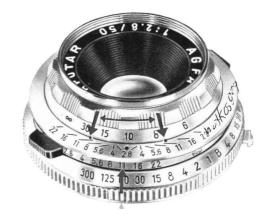
If the camera is focused on 10 feet the sharp zone will be from about 8 to 20 feet. In the above illustration arrows and dots have been included to make this point clearer and show how you can read off the depth of field from the focusing scale of your camera.
