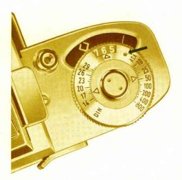
film first look for its speed rating on the carton and set this on the ASA/DIN scale. If your film is rated by another system the comparative table on the opposite page will give you the corresponding value. To set the speed turn the inner scale ring by the projection (see arrow) until the required figure is opposite the triangular mark. Our illustration shows a film speed setting of 40 ASA (17° DIN).
