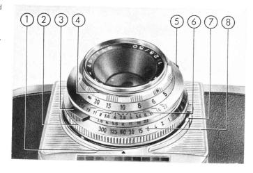
The green numbers on the shutter speed ring cannot be set but merely indicate the correct length of time exposures on the "B" setting. For further details see pages 18 and 19.
